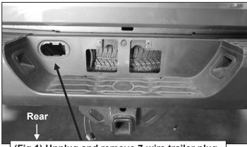
(Fig 1) Unplug and remove 7-wire trailer plug
