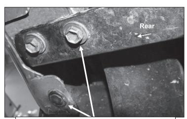
(Fig 5) Remove Factory Hardware and Plastic Clip from the underside of the bumper
