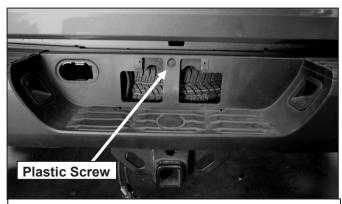
(Fig 4) Remove plastic screw previously under the license plate.
