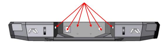
E. Install bumper mounts onto bumper as shown using supplied mounting hardware: bolts, washers, and nuts. Do not tighten fully. Verify that the triangular flange points upward and middle flange faces outward. Repeat for other side. See Image Below.
