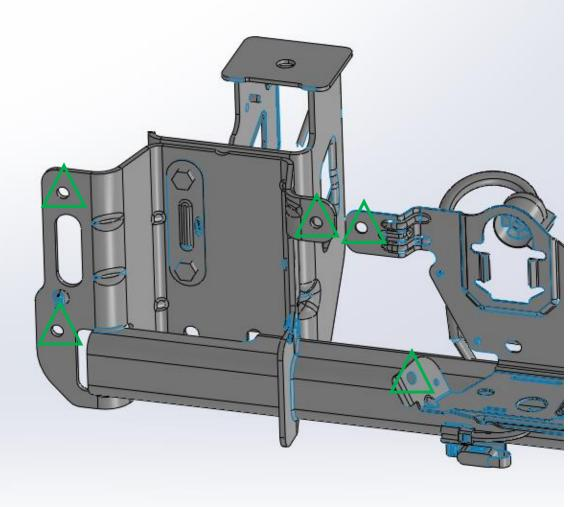
Figure 4c (5x Bolt Locations Per Side)
