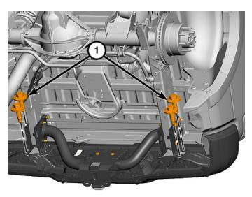
4. With assistance, remove the bumper from the truck. Using a 10mm socket wrench, remove the two (2) bolts and support plates from the frame rails on both the driver and passenger side. (Figure 4, #1)
