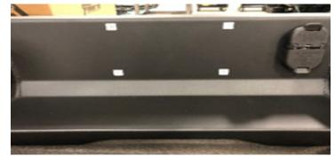
29. Insert the provided four (4) nylon license plate nut inserts into the four holes on the bumper. (50189-HW) (Figure 27)
