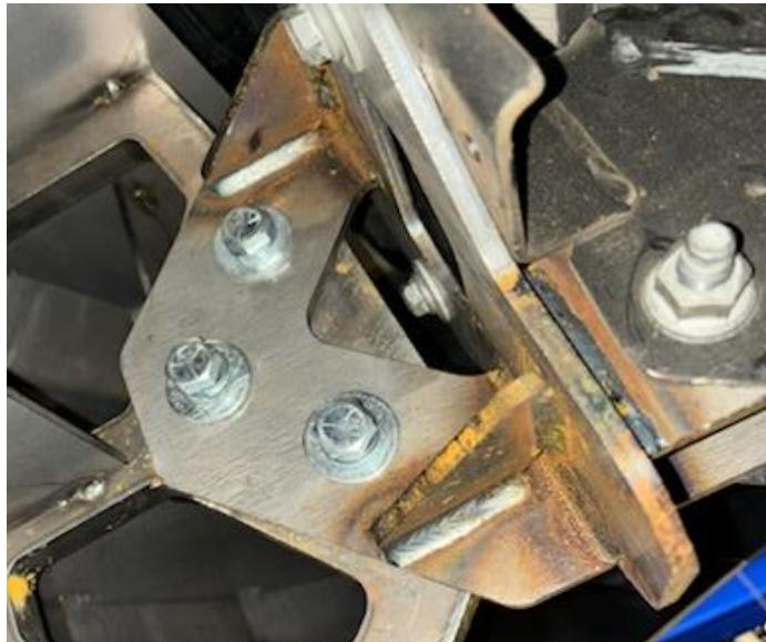
3. Once all bolts are started, push the bumper back against the vehicle and tilt the bumper forward to ensure an even spacing between the bumper and the vehicle. Using a  $\frac{3}{4}$ " socket, tighten all the bolts to the recommended torque specs listed. (Page 2)
