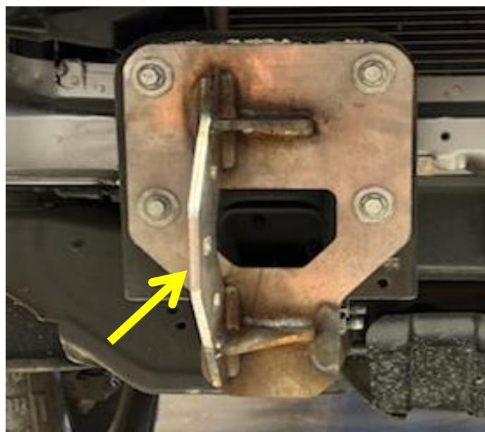
2. Using a hoist, align the bumper slots with the frame mount slots. Once aligned, place the top and bottom bolts through the slots with a weldnut tab D on the inner part of the plate (driver side shown). Start the top bolt but do not tighten, install and tighten the bottom bolt using a  $\frac{3}{4}$ " socket. Tilt the bumper forward and install the middle bolt.
