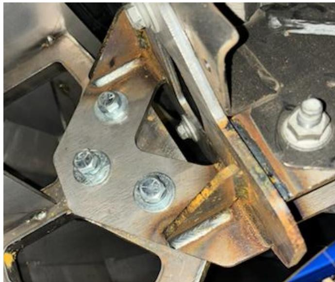
3. Once all bolts are started, push the bumper back against the vehicle and tilt the bumper forward to ensure an even spacing between the bumper and the vehicle. Using a  $\frac{3}{4}$ " socket, tighten all the bolts to the recommended torque specs listed. (Page 2)
