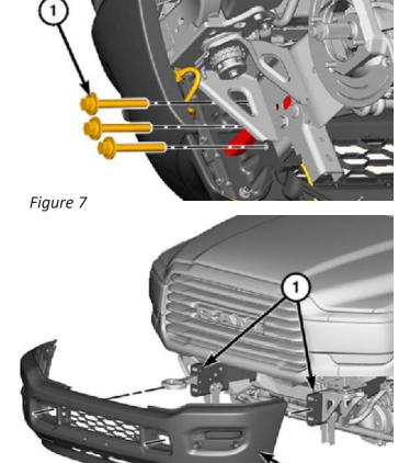
9. Using a 24mm socket wrench, remove the factory bolt and nut tabs from the frame rail to remove the factory tow hooks and crash bars. (Figure 9)
