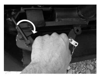
B. Your tire carrier is equipped with a retaining pin that will hold your tire carrier open when getting items in and out of the back of the vehicle. It, however, is not to be used as a catch for swinging the tire carrier opened uncontrolled for it to engage. Any uncontrolled opening could result in damage to the tire carrier itself, the bumper, and possibly the vehicle it is installed on. PLEASE USE CAUTION WHEN OPENING!
