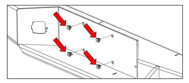
Figure 7 – License plate nylon nut insertion
