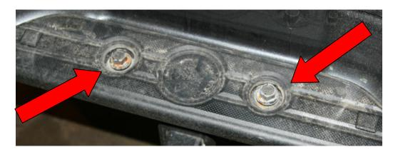
Figure 3 – Trailer hitch bolt removal
