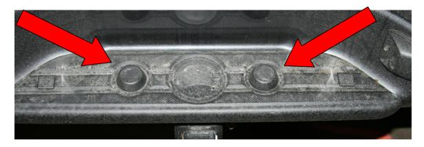
Figure 2 – Bolt cover removal
