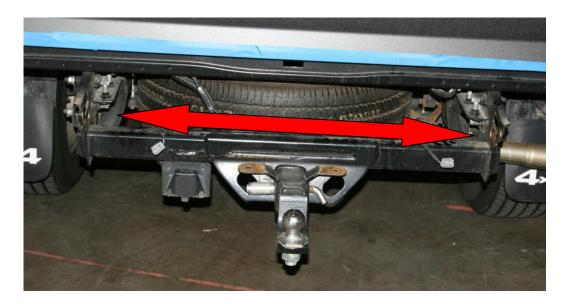
Figure 5 – OEM mounting plates may need width adjustment
