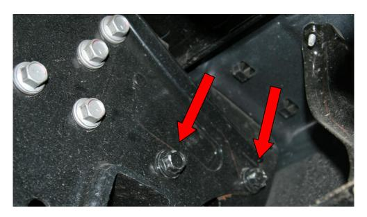
Figure 4 – OEM bumper bolt removal
