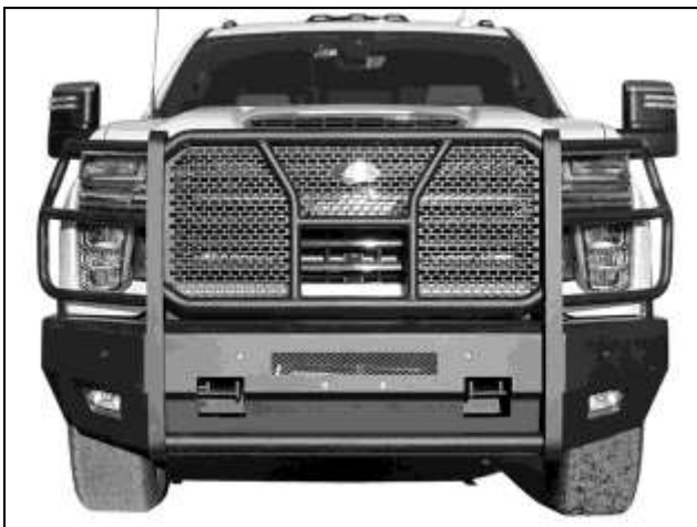
(Fig 29) Attach passenger/right fog light to mounting tabs on driver/left side of Bumper
