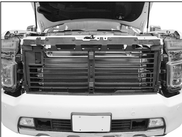
(Fig 7) Grille and fascia removed
