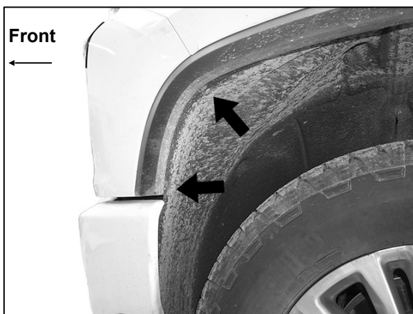
(Fig 1) Release hardware attaching fender liner from plastic panel (fascia-see arrows)
