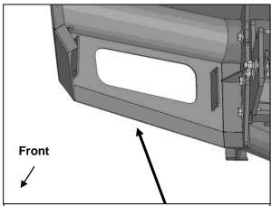
(Fig 22) Remove fog light mount from back of Bumper (driver/left side illustrated)
