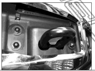
(Fig 5) Remove bumper bolts (driver side pictured)
