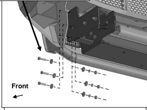
(Fig 15) Attach Bumper to side of Bracket
