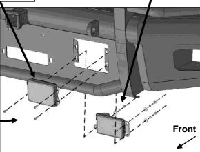
(Fig 14) Attach "Early" ACC and plastic cover to the ACC Brackets
