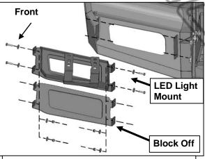
(Fig 23) Models with LED fog lights only, reuse screws to attach LED fog light to Light Mount.
