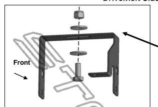
(Fig 17) Optional OEM fog light installation (light not included). Attach driver/left Upper Bracket to the slot in top of the opening
