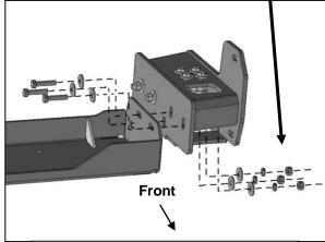
(Fig 9) Attach Winch Tray to Bracket
