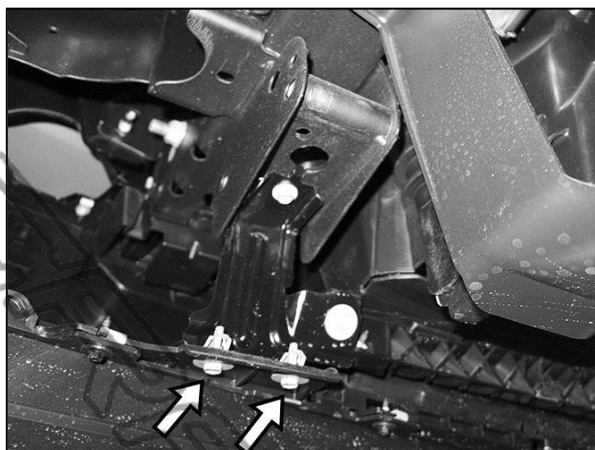
(Fig 8) Remove bolts attaching bottom of bumper to brackets (arrows). Driver/left side pictured
