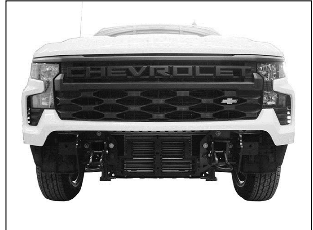
(Fig 24) Reinstall fascia body panel, grille and cover. Reattach inner fender liners
