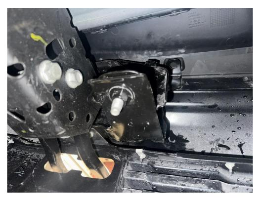
12. Using a 15mm socket, remove three bolts attaching the side brace to the bumper/frame. Remove and set aside as it will not be reused. (Both sides)
