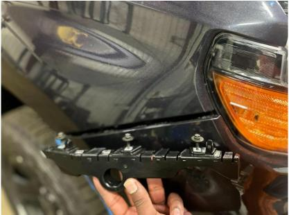
5. Carefully pull out on the grill side panel until separated from truck's face and grill.
