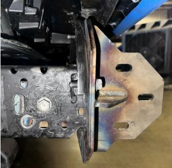
4. Using a hoist or a few helpers, lift the bumper onto the frame mounts and attach using hardware kit #58 and weldnut tab D. Start all bolts before aligning bumper. Ensure the bumper is pushed back as far as possible and snug bolts with a <sup>3</sup>/<sub>4</sub>" socket or wrench.
