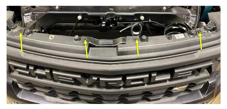
8. Using your hand, pick up on the top of the grill and pull away from the truck. This will disengage tabs on the top of the grill and allow its removal.
