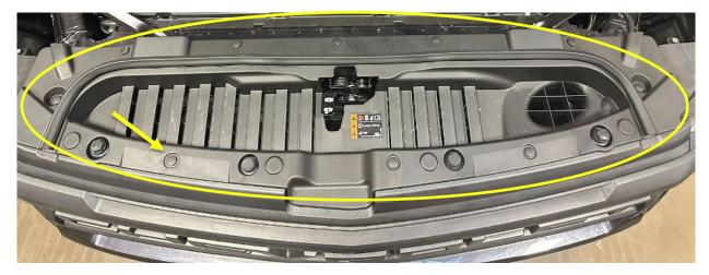
3. Using a T-15 bit remove four screws holding the fender liner in place.(Both sides)
