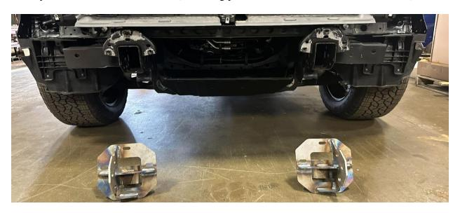
2. Install frame mounts using OE hardware as shown. Do not fully tigbhten.
