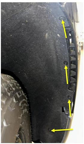
4. Using a 7mm socket, remove the three screws attaching the grill side panel to the body. These screws will be more accessible from inside the hood of the truck.(Both sides)
