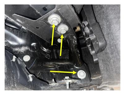
13. Using a 10mm socket, remove the bolt attaching bottom brace to bumper/frame. Remove braces and set aside. It will not be reused. (Both sides)
