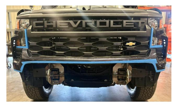
3. Insert OE long bolt from tow hook throught the side hole located on the frame. Fully tighten all frame mount bolts.
